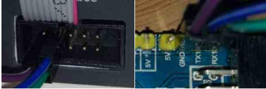
Figure 2.2 The connection between Dobot Magician and the development board
